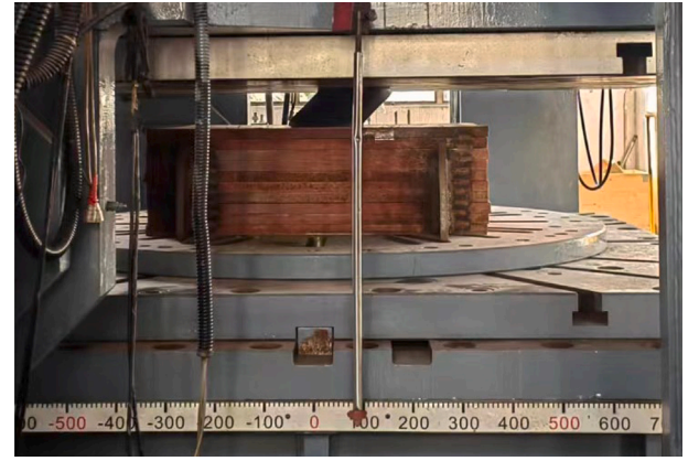
Fig. 7. Horizontal quasi-static hysteresis test on the isolation bearing.
